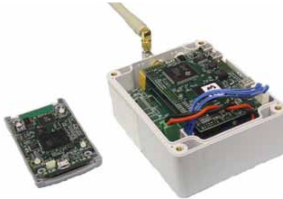
Figure 1: WASP node hardware, with tag on left and base station on right.
