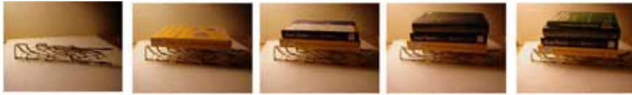
Figure 9. Load testing on the interwoven stress lines
