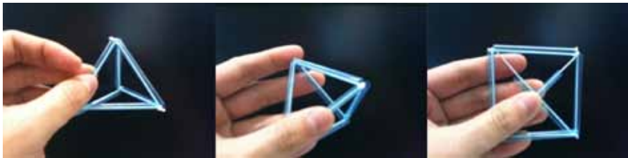
Figure 2. Elastic Tetrahedron is formed by elastic string and plastic hollow straws for their lightweight and flexible purpose.
