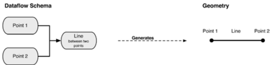
Figure 1. Left: A schema as a directed acyclic graph. The data from the two points flows to the line node informing its construction. Right: Geometry that results from schema on left.
