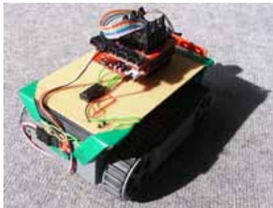
Figure 1. An implementation of Braitenberg Vehicle.
