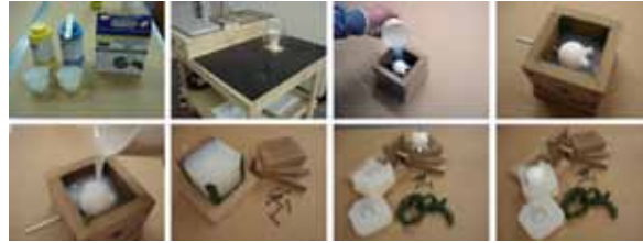
Figure 6: Mould making and casting process
