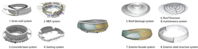
Figure 2. Eight systems for the hybrid building
