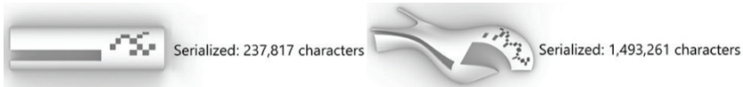
Figure 1: Geometry text representation: the length of the serialized text for the more complex geometry is six times longer (heavier) than that of the simple geometry
