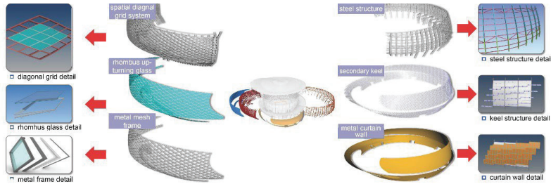
Figure 3. Exterior curtain wall system of the stadium
