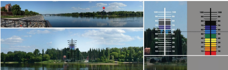
Figure 3. Simulation of the planned tall building with the view from the riverfront. The simulation uses a height ruler and every 10 m colour coding for the facility
