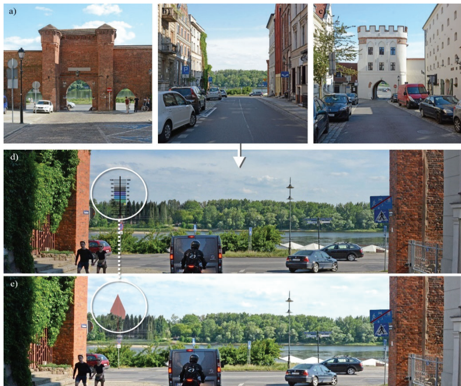
Figure 5. Axial exposure from the streets of the old town towards the river and the planned tall building (a, b, c); d) simulation of the tall building and a height ruler (building height 85 m); e) simulation of the building slender towards its top; colour of the tall building is a reference to brick facades of the old town (building height 100 m).
