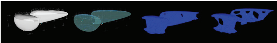
Figure 4. BESO analysis result of prototype X and Y together in Ameba (Zhou et al., 2018): (a) initial design mesh with force analysis from CFD; (b) force analysis with mesh structure curves on; (c) topological optimization in progress, (d) the result of topological optimization.
