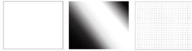
Figure 3. (left) 500*400mm (width * height) panel area; (middle) gray-scale sample image; (right) original point grid.
