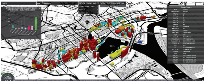
Figure 5: UDT dashboard showing the GHG emission query result for commercial buildings in the
