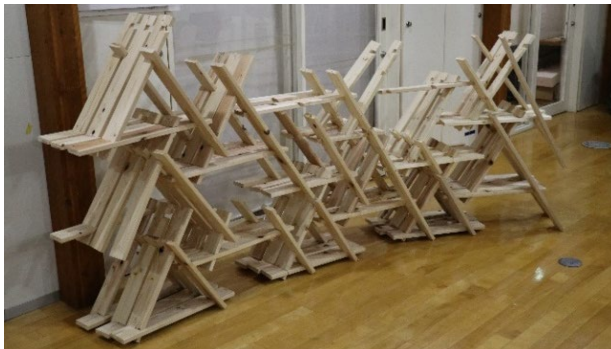
Figure 1. Fabricated shelf structure
