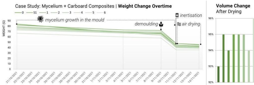
Figure 3. Weight (left) and volume (right) change overtime: 'Cardboard Composites' study
