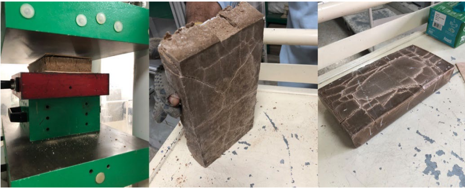
Figure 6. Strength of material testing, result of sand brick after normalized compression test.
