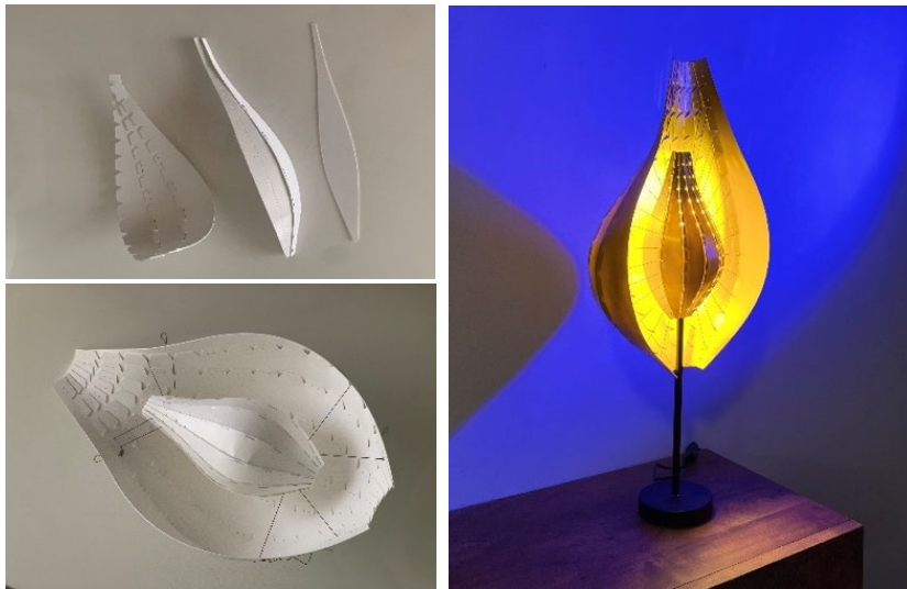
Figure 5. (top left) Partially assembled shells for fabricated panels, (bottom left) completed shells joined with Kevlar fibre and tested for maintaining structure, (right) Finished lamp design.
