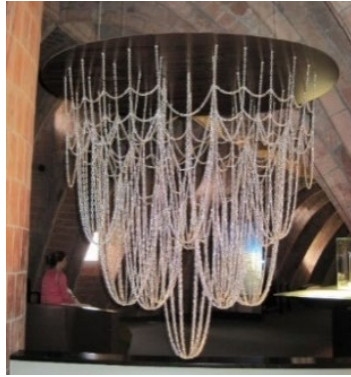
Figure 1.1 Antonio Gaudi's chain model hanging in the Sagrada Família
