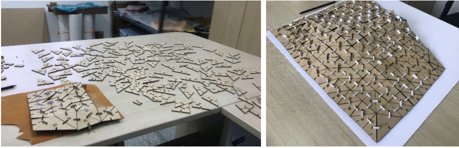
Figure 6. MDF prototype in 1:10 scale of the auto-meshed trapezoid geometry '2a'
