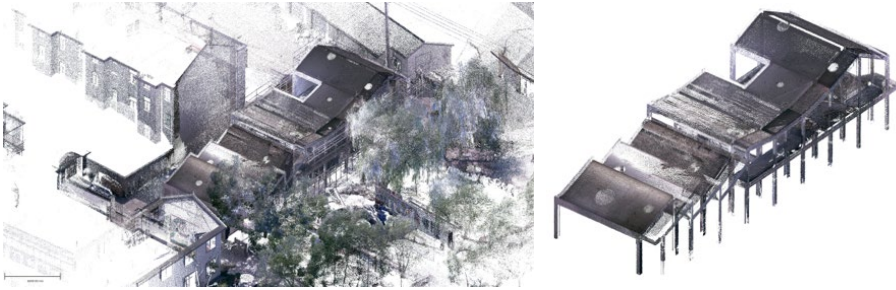
Figure 5. Registered point cloud of the building (left); Figure 6. Extracted structural point cloud model (right)
