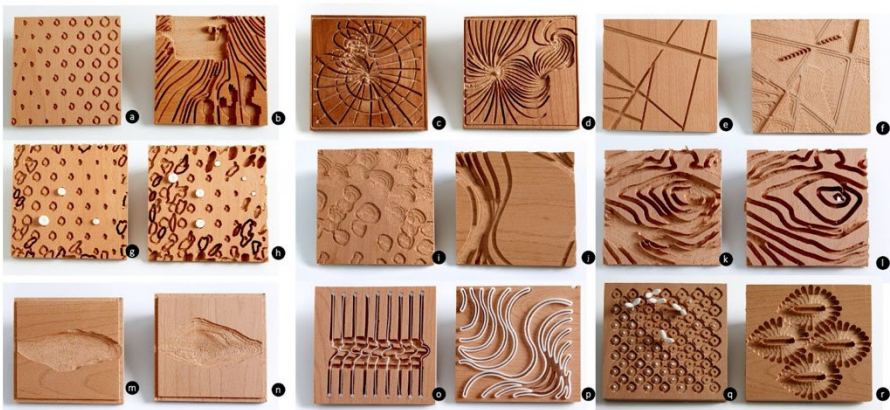
Figure 5 Sample collection of patterned texture that communicate botanical, geographical or marine data for touch access, including hybrid objects (subtractive/additive manufacturing coupled).
