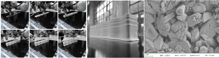
Figure 9. Print process and micro-structure of gypsum treated with modified components
