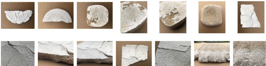
Figure 3. Material tests using sand and sodium to create bio-synthetic sandstone
