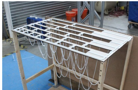
Figure 2.2 Completed material draping test over wooden profile template.
