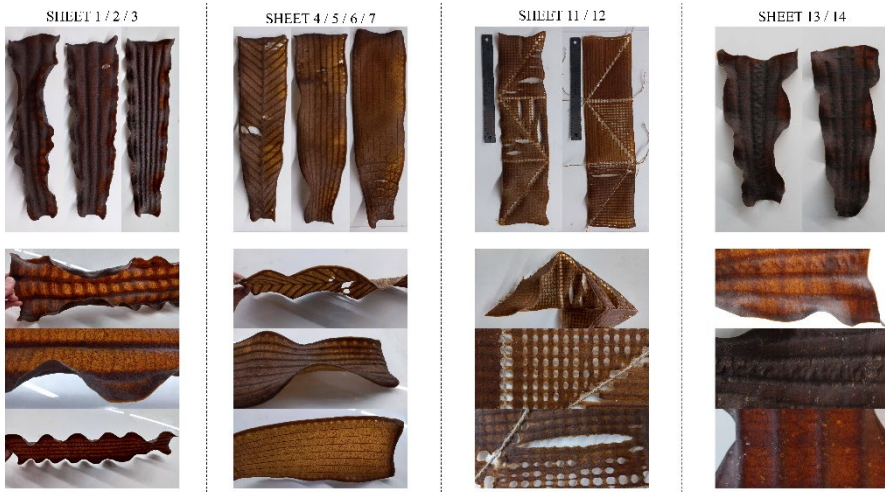
Figure 4. Catalogue of Robotically Extruded Multi-layered Sheets
