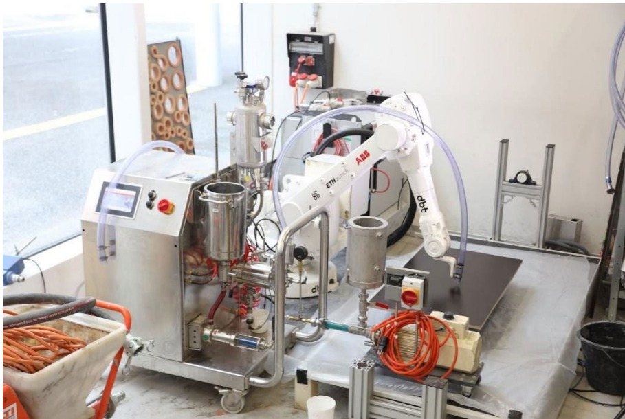
Figure 1. The robotic F3DP setup with the stationary foam generator in the foreground connected to the industrial robot in the background.
