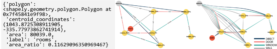
Figure 11. Left: The key value pairs of all property information of a room node in JSON format; Middle: A simple-attributed graph sample; Right: A multi-attributed graph sample
