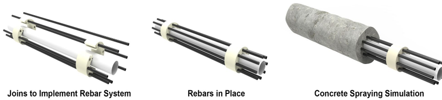
Figure 2. Construction System - PVC Pipes/Rebars/Joins
