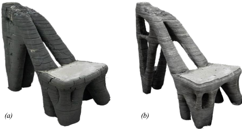
Figure 8. The final artifact of the tree support: (a) the clay mould a day after the final cast (before demoulding); (b) the concrete prototype (after demoulding).
