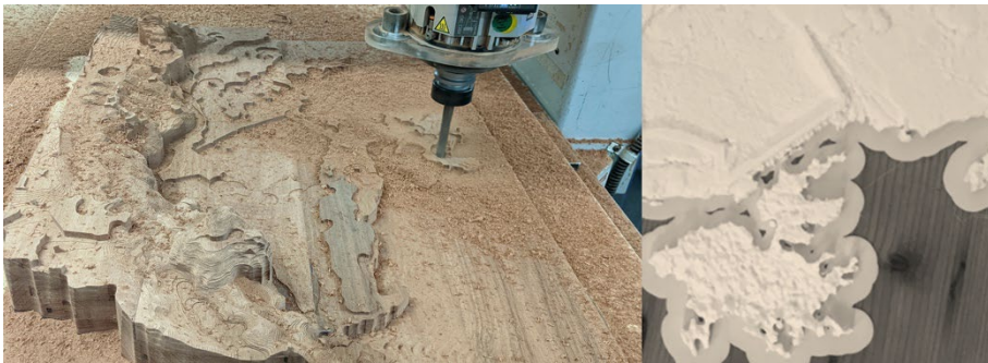
Figure 3. Malabar Ocean Pool | CNC milled timber model with benches and 3D prints (PVC)
