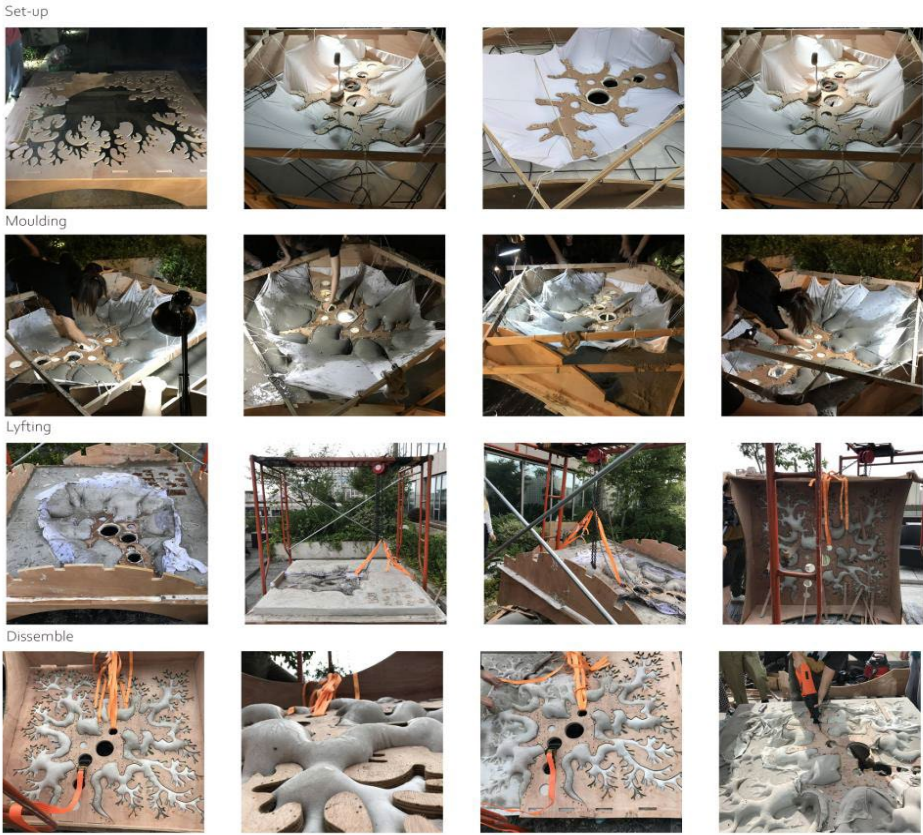
Figure 8. The fabrication process
