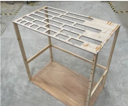
Figure 2.7 Profile template #1 with inconsistent edge conditions on the right side.
