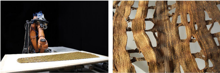
Figure 5. Large-scale Printing using the Kuka Robot (left) and Dried Results (right)
