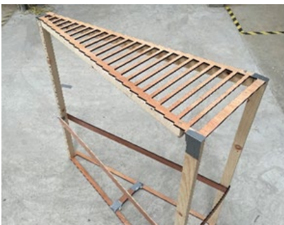
Figure 2.9 Profile template #2 with a one-inch edge condition.
