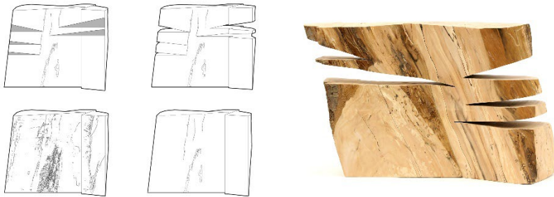
Figure 9. Using edge detection to locate cracks and mill wedges. Work by Stuart Ingram
