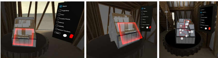
Figure 7. Images showing the miniature inside the building. The user can see the insides by manipulating a clipping plane (shown in the left and middle images). The right image shows the keypoints and trajectory as well.
