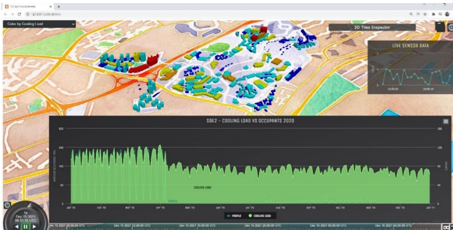
Figure 7. Digital twin dashboard showing the cooling load scene
