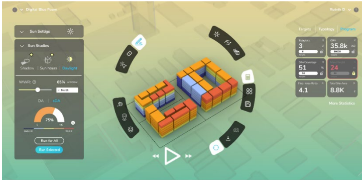
Figure 5. DBF building DA prediction system is based on ML and dramatically reduces daylight analysis time compared to traditional simulation-based approaches. The building score is given on the UI. The building parts performance is represented as coloured units visualized on the 3D model
