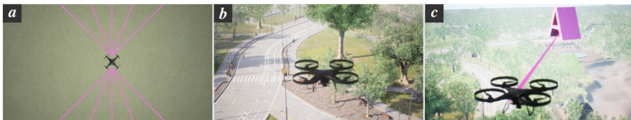
Figure 3. (a) Distance detection system (b) Third-person perspective (c) Path planning
