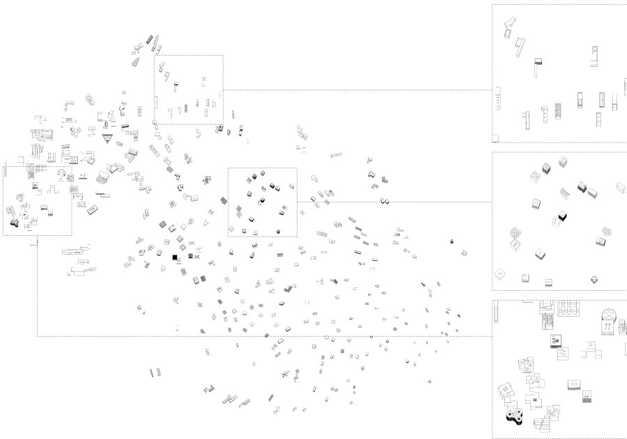
Figure 7. t-SNE plot of machine-learned forms using 'architectural' point clouds at 9,000 epochs with close-ups of clustering of different formal groups.
