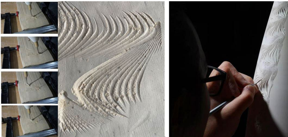
Figure 10. Comparison between the results details of robotic engraving and traditional carving craft
