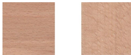
Figure 4. (Left) Spindles formed by the medullary rays run mostly parallel to the annual growth ring. (Right) Spindles formed by the medullary rays running mostly at an angle of 315° to the annual growth ring.
