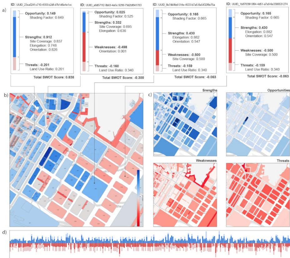
Figure 4 shows one of the four regions SWOT analysis results: a) presents the score composition of four example plots; b) visualises the distribution of total SWOT analysis results; c) maps visualise the distributions of separate descriptors. Concentrations of S and O primarily consist of developed plots with high-rise buildings, while W and T cluster in areas that are not yet developed; d) displays a bar chart with SWOT results for all plots, showing that most plots balance negative and positive factors and that only very few plots are highly suitable or highly unsuitable for PV installation.
