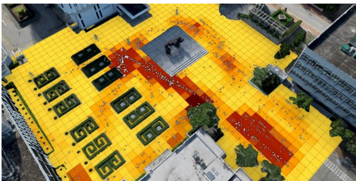
Figure 7: Space-centric analysis of people locations and closeness, based on the combined pedestrian location data of 8.5 minutes of drone scanning
