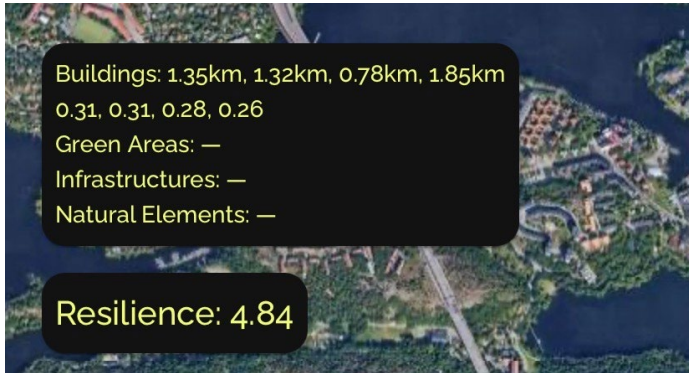
Figure 6. Screen grab of the app showing the overall value R and 4 clusters of buildings detected by the model. The distance from the centre of the area to each cluster is used to calculate the individual contribution of that cluster to R (0.31, 0.28, 0.26).
