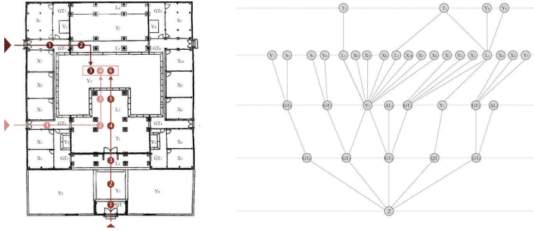
Figure 3. (left) the plan of house in Jinyun, Zhejiang (right) automatic generated justified map.
