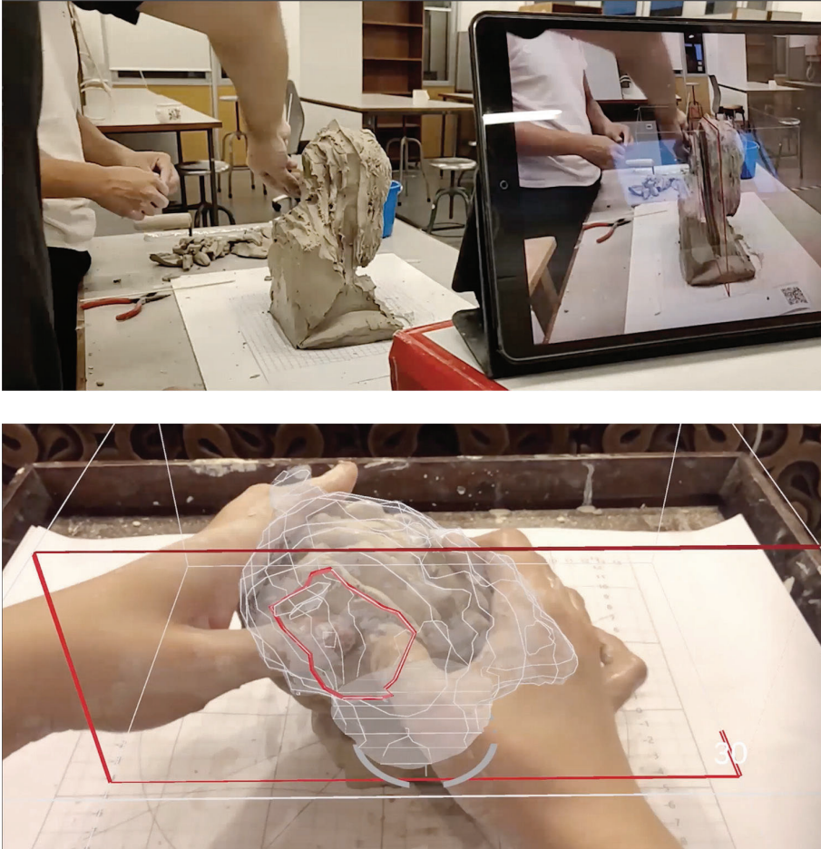
Figure 6. Top: View through mobile device with holographic instructions and view on clay model where mass is removed or added accordingly. Bottom: Sculpting while viewing through mobile device with holographic instructions. .
