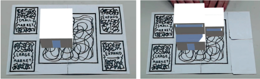
Figure 3. Image-based target, with two virtual buttons on either side of the central tracker. Covering the ‘expand up’ and ‘expand out’ virtual buttons causes a new typology to be created.
