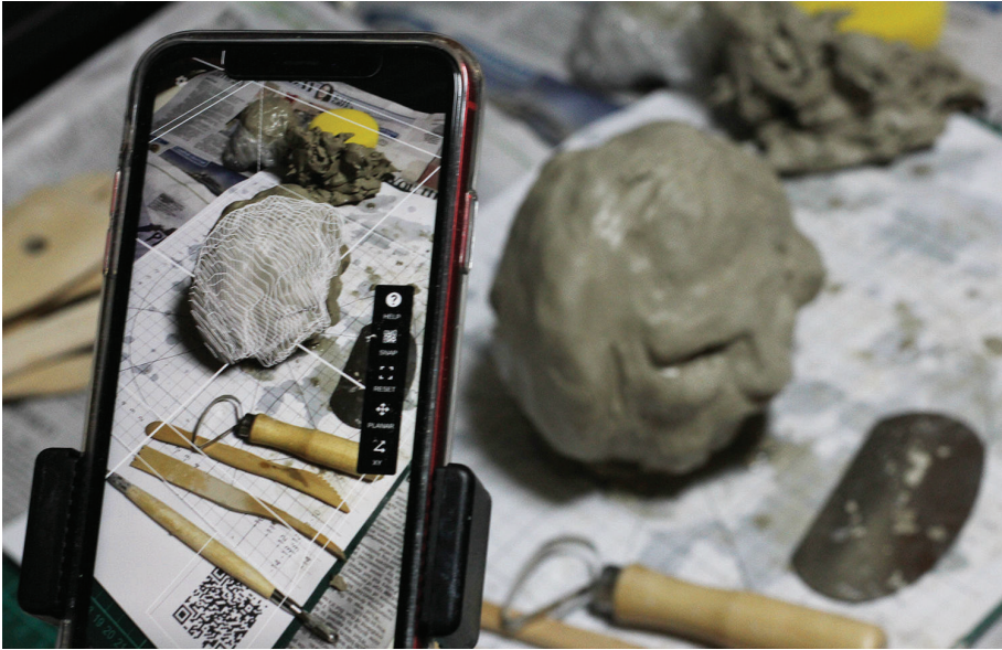
Figure 4. View through smartphone of customised AR application, showcasing the overlay of holographic instructions on top of the physical clay model.
