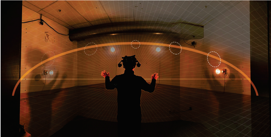
Figure 5. Mixed Reality demonstrating the sun's path of travel around the user, with heat lamp connection.
