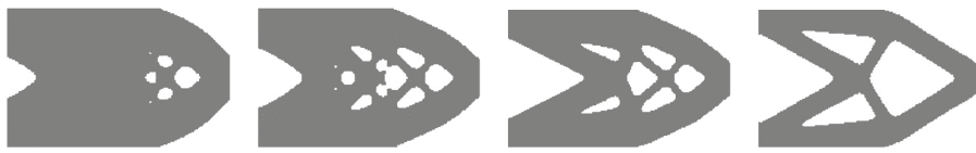
Figure 3. Bi-directional Evolutionary Structural Optimisation (BESO).
