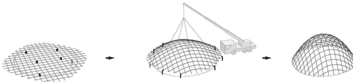
Figure 2. Deployable “flatbed” structures prefabricate an initially flat regular grid with no shear rigidity and elastically deform and brace it into place.
