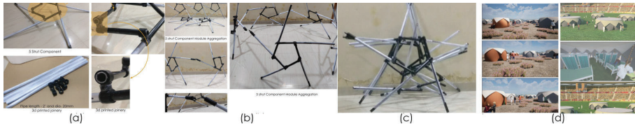
Figure 12. (a): Construction of Component. (b): Construction of Aggregation Unit (c): Deployed form. Scale Prototype (Source: Author) (d): Visual Representation (Source: Author).
