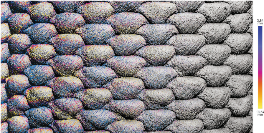
Figure 7. Distance-based comparison between a 3D scanned C3DP column and its 3D digital model designed through toolpath manipulation.
