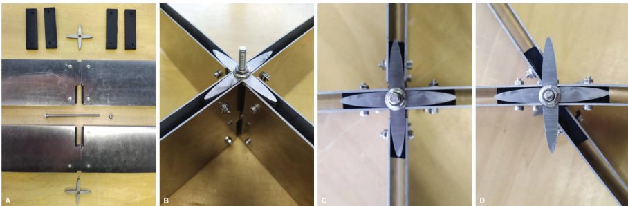
Figure 4. Composite joint system from two 1.5mm stainless steel strips with 8mm rubber inlays (A). The joints are designed to allow up to \pm 30^\circ rotation freedom during assembly (D) and lock at 90 degrees once the rounded star-washers are fixed (B, C).
