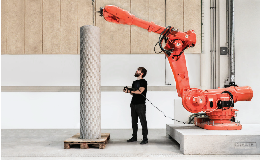
Figure 6. Concrete 3D Printed hollow column presenting an alternated XY toolpath manipulation.
