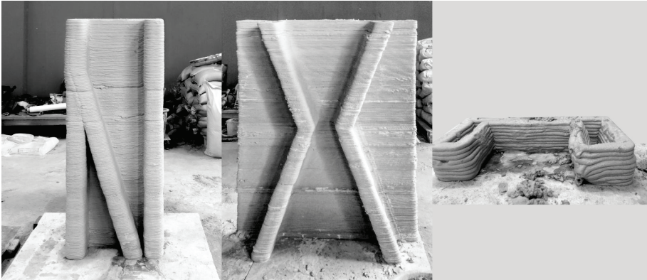
Figure 4. incline angle test 15°(left),20°(middle),25°(right).
