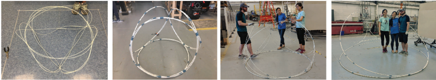
Figure 5. Figure 5. (L-R) 5A: 1/6 scale model (left); 5B: 1/4 scale model from 2 No.1/4" diam. rods; 5C: 1/4 scale model from 2 No.3/16" diam. rods; and 5D: full-scale 'pringle' model (right).
