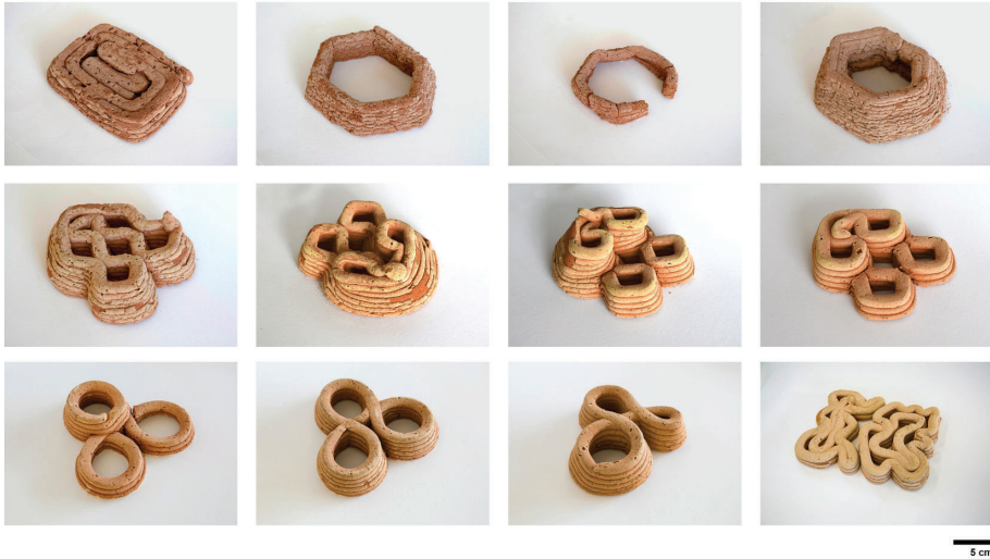
Figure 2. Prototyping evolution. Top row: improving surface quality. Middle row: maximizing print height. Bottom row: reducing cracks.
