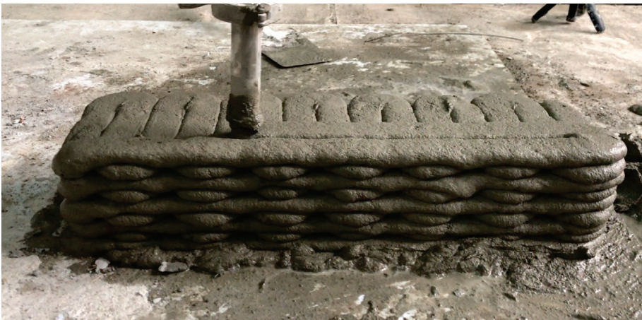
Figure 5. 90° cross pattern of test sample.
