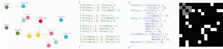
Figure 4. Plan 41: Graph, Triplet, Adjacency List and Adjacency Matrix as Rasterized Image.
