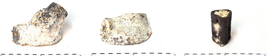
Figure 4. Inoculated node (left, middle) and bar (right) elements after 14 days of growth.
