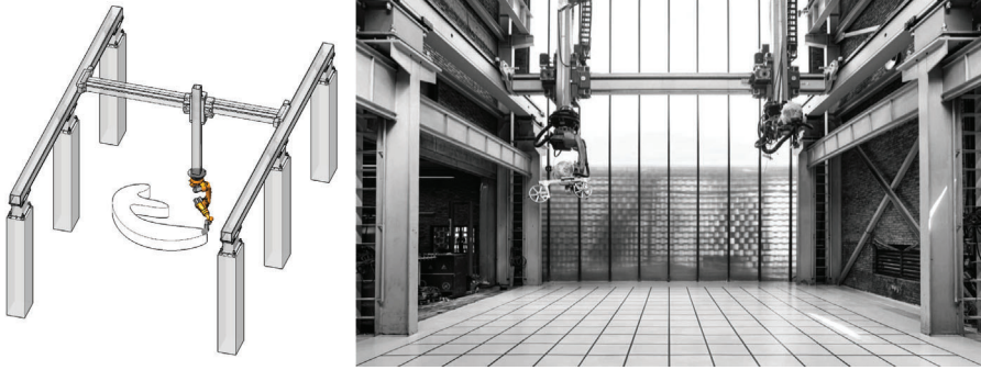
Figure 6. XYZ external axis.
