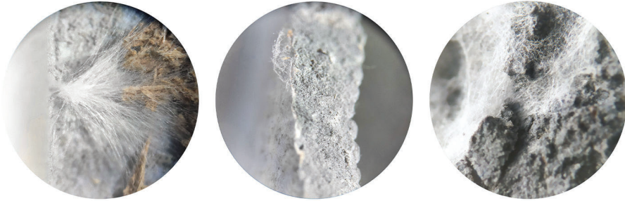
Figure 3. Mycelial advancement through the 3D printed clay wall (9.5 mm) at 20x magnification (left). Surface growth on a 3D printed clay wall (2.5 mm) at 20x magnification (middle). Hyphae connection between two elements at 30x magnification (right).
