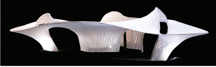
Figure 11. Final 1:20 scale physical prototype (2.4m x 2 m x 0.5m).
