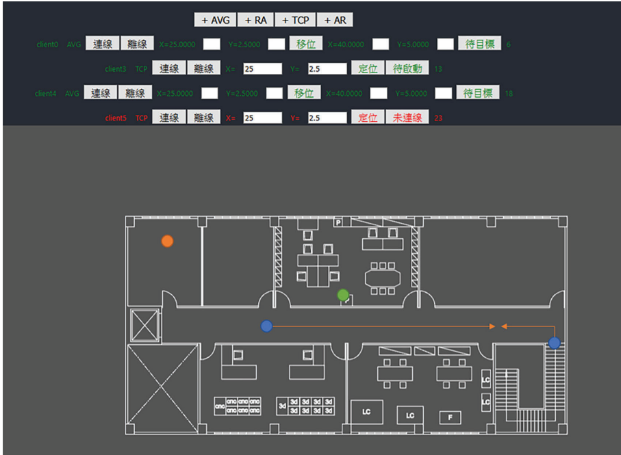
Figure 5. The FOS represents the node communication result via monitor ROS master and graphical remapping of the allocation of nodes.
