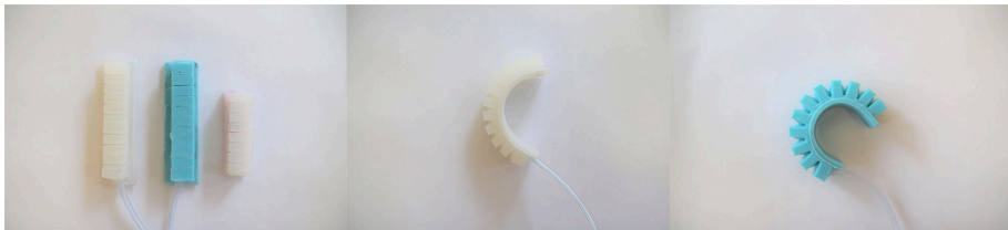
Figure 2. Example of Platsil Gel 00-30, Mold Star 16A, Platsil Gel 00-10, (Left to right).
