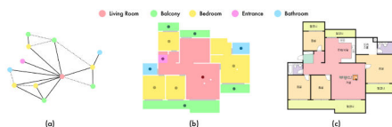
Figure 1. Three types of references with different LoD (a) Abstract (b) Hybrid (c) Concrete.
