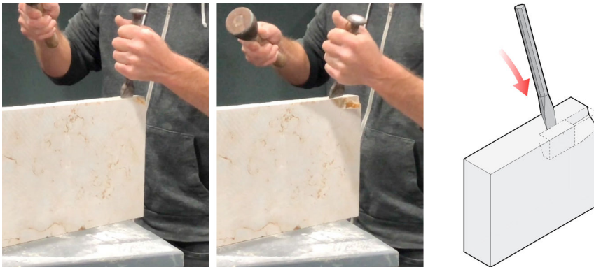
Figure 2. The stone carver removes the sharp edges of a sawed stone in preparation for surface processing. In this example, the human eye notices the amount of material subtracted in the previous action. That knowledge guides the craftsman's decision regarding where to place the tool for the following action (MTRL, 2019).
