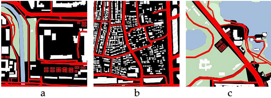
Figure 2. Coloured labelled map, red: road; green: green land; blue: river; white: building; black: empty; a) common city map with all elements; b) condense city map with only roads and buildings; c) loose city map with large green lands and rivers.
