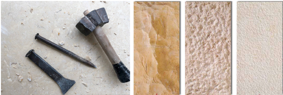
Figure 3. (left) Traditional stone carving tools and (right) examples of stone dressing techniques as classified by T. Canaan (1933): ruscated (Tubzeh), coarse (Taltish), and pointed (Musamsam). Photo taken at A.Grebelsky & Son (MTRL, 2019).
