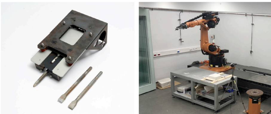
Figure 7. The toolkit: (left) a custom multi-tool end effector; (right) the robotic cell - including a KUKA KR60 robotic arm mounted on a KL1000-2 linear rail, an XY positioning table, and peripheral cameras (MTRL, 2019).
