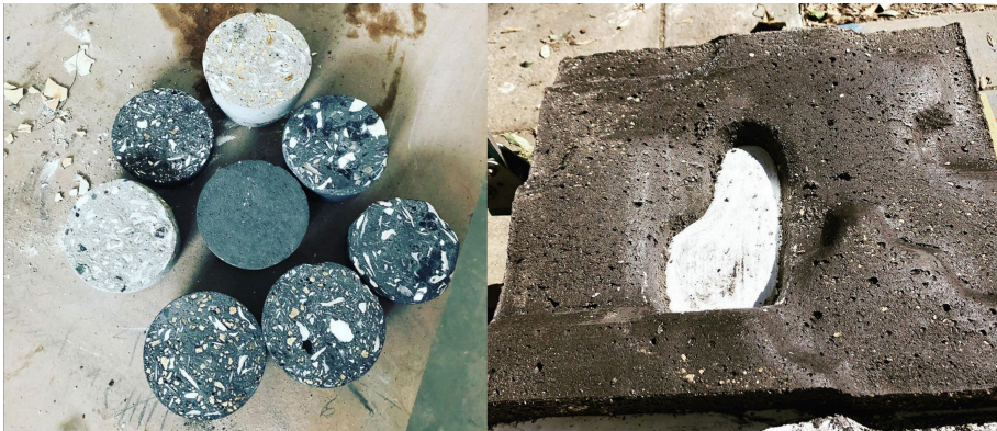
Figure 6. Hybrid material composite samples made of concrete and crushed discarded oyster shells then used for the large prototype piece (Dunn 2019).
