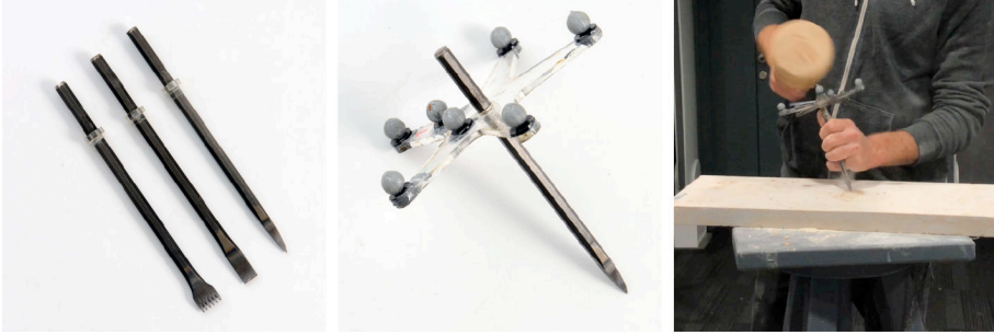
Figure 4. The chisel mounted with an adapter that is tracked to produce the tool's position and orientation throughout a carving session (MTRL, 2019).
