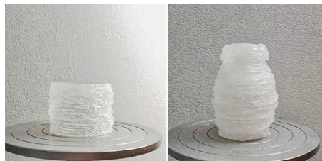
Figure 6. Vases printed by PICA.
