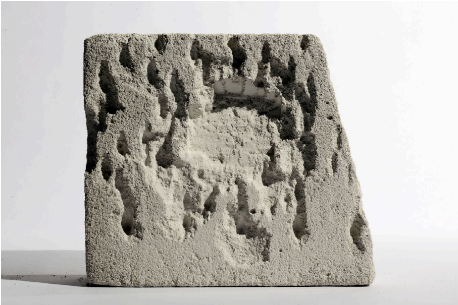
Figure 1. An autonomously produced robotic element based on traditional, region-specific stone carving techniques (MTRL, 2019).
