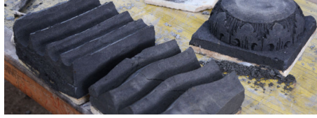
Figure 2. Image showing carved test pieces with ruled surfaces, and a single convex surface.
