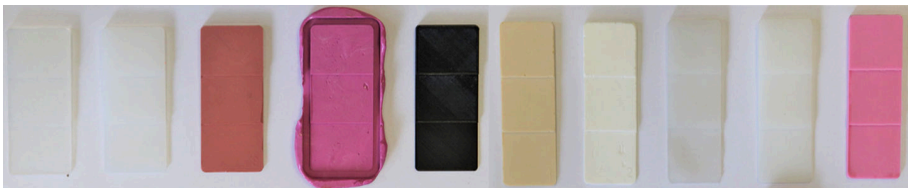
Figure 1. A range of silicones tested based on their Shore Hardness ranging from 00-10 to A90.
