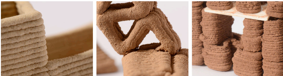
Figure 3. Printed samples of architectural details using the various sands available on-site. Work by students Elena Tabakova, Hala Hamzi, and Noa Gigi (MTRL, 2019).
