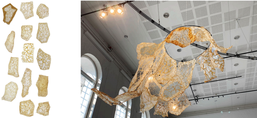
Figure 7. First generation of robotically fabricated panels and mock-up for assembly test. .
