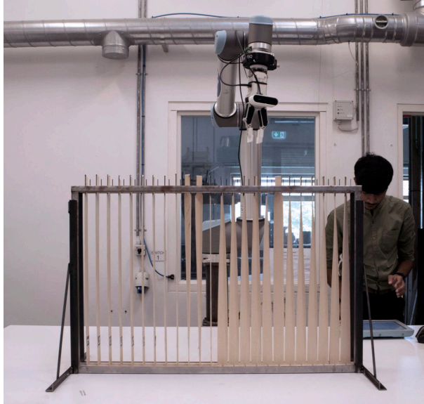
Figure 3. The physical design system consist of 24 wood lamellas mounted in a steel frame. Variations caused by rotation of individual elements creates potential for directed views and intentional blocking of sunlight.
