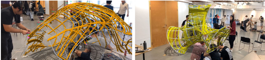
Figure 9. Densification of components guided by holographically overlaid flow patterns.
