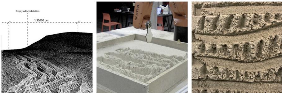
Figure 6. Exploring large-scale construction: using robotic tools towards remotely forming lunar structures with the given topographical conditions. Work by students Meriem Benkirane, Maelle Kolimedje, Charles-Edgar Lincoln, and Jihla Prentis (Confluence Institute, 2019).
