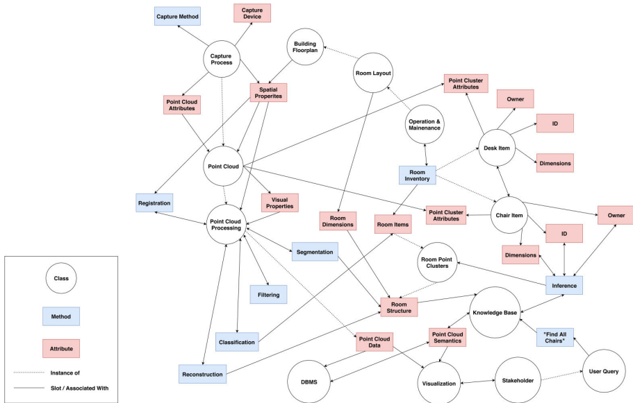
Figure 2. A core ontology example for using a point cloud representation for an O&M task.
