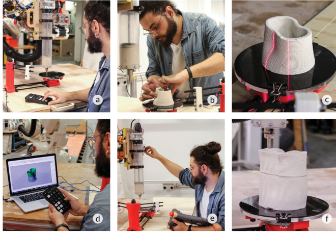
Figure 3. Stages of an exemplary use case scenario: (a) initiating the fabrication, (b) physical deformation of the artifact, (c) 3D capturing of the modified artifact, (d) user conforming design hypotheses, (e) user controlling the extrusion rate, (f) finished extrapolated geometry.
