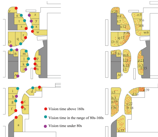
Figure 7. Comparison of vision focuses simulation results (left) with the commercial space vitality survey results (right).
