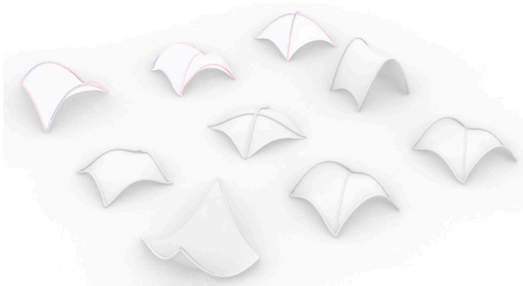
Figure 4. Simulated outcomes generated using Grasshopper and Karamba 3D definition.
