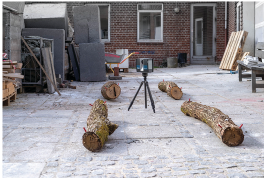
Figure 2. Figure 2 Scanning of the logs are currently performed using a lidar scanner; however, multiple techniques have been tested and tried. These logs are scanned on the ground, while later tests showed that the scan data was improved when placing the logs on stands.
