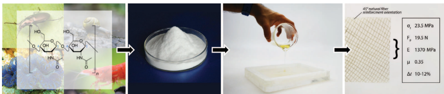
Figure 1. A simple schematic transformation of raw chitosan into thin films.
