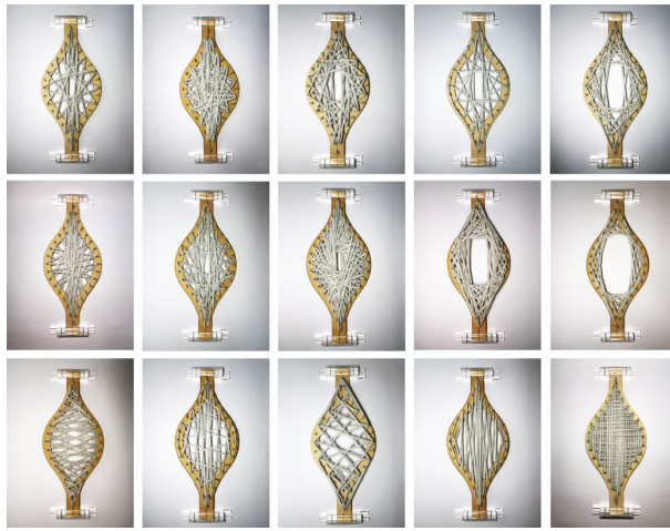
Figure 9. Winding PET fiber with robotic arm.
