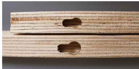
Figure 3. 13mm Mortise vs 16mm Mortise.
