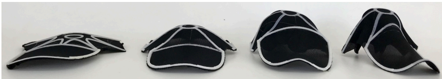
Figure 6. Evolution of a functional prototype. From a planar form (right) to the three-dimensional prototype (right) generated an increase in height after tension was released.
