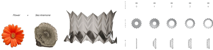
Figure 4. The blooming of a flower and sea anemone (left) combined with origami folds (center) inspired this blooming flower-like form for a facade surface (right).
