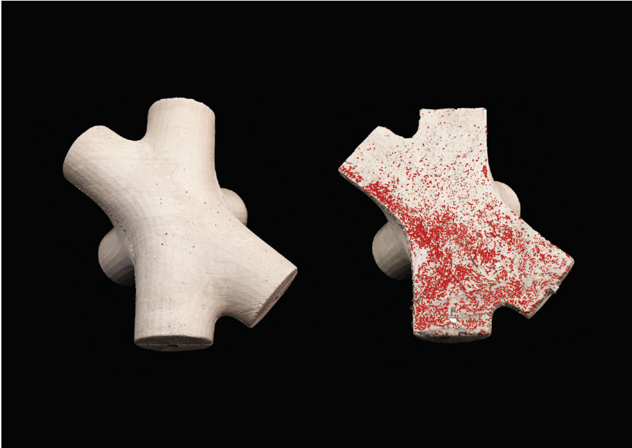
Figure 7. Analysis of the steel fibres distribution occurring through a vertical section of the node.
