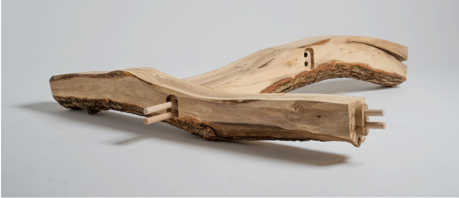
Figure 6. Two curved logs joined together using the developed workflow. The two logs describe a part of a larger surface.
