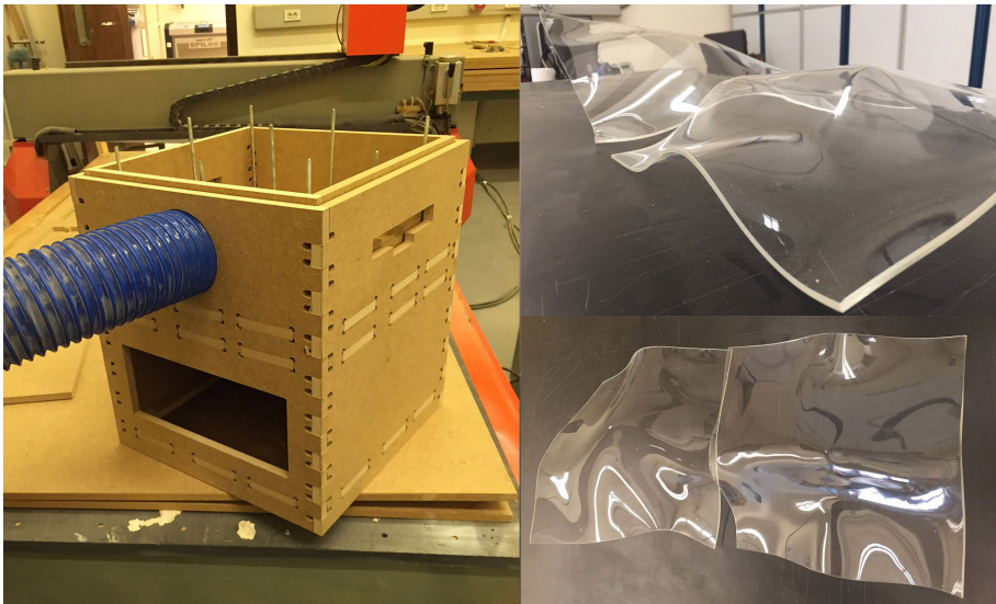
Figure 3. Vacuum forming output (Left: Vacuum forming device based on multipoint forming and material deposition, Right: Fabricated acrylic tiles).
