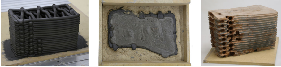
Figure 5. Fabrication Procedures. (a) Printed clay mould. (b) Sandbox reinforce the concrete casting. (3) Demoulded concrete block.
