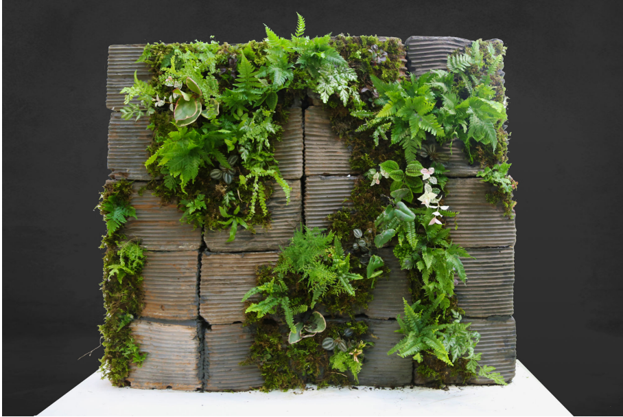
Figure 7. Integrated concrete green wall made of twenty segments.
