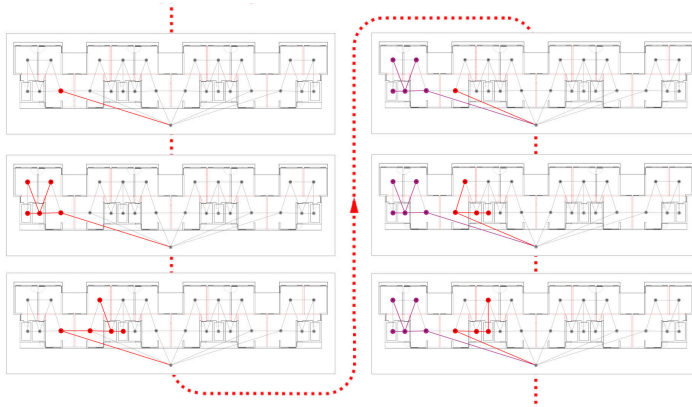
Figure 8. Example of node traversal and unit allocation in the algorithm. Traversal path is shown in red; once it is defined as a unit (shown in purple), the algorithm tries the next path traversal for another unit.
