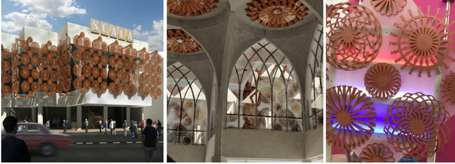
Figure 6. Theater performance facade project using spinning flower shape patterns that double as visual performance elements and a ventilation fan.
